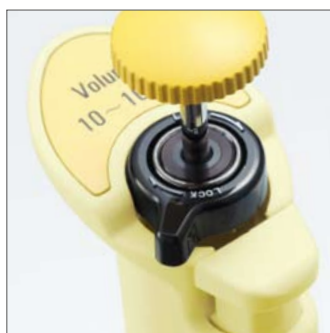
Easy calibration with enclosed jig
